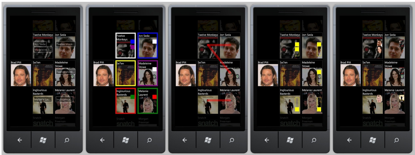
Figure 1: Different explicit link representations for GraphTiles . (a) text : nodes with the same name are linked. (b) color : nodes with the same color are linked. (c) connectedness : nodes with lines between them are linked. (d) proximity : nodes at/containing the same vertical position are linked. (e) texture : nodes with/containing the same image are linked.
