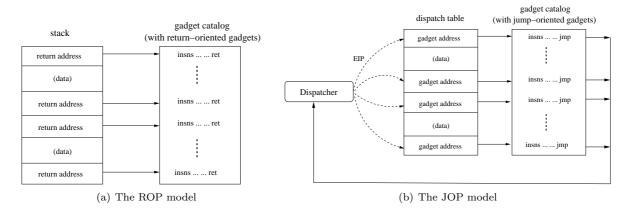
Figure 1: Return-oriented programming (ROP) vs. jump-oriented programming (JOP)
